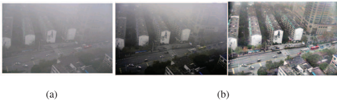
Fig. 7. Here we show some contrast enhancement comparison results. In Fig 7(a) we show the input image. In Fig 7(b) the contrast enhancement result using the normal global contrast enhancement method (the left figure) and our proposed algorithm (the right figure) are compared.
