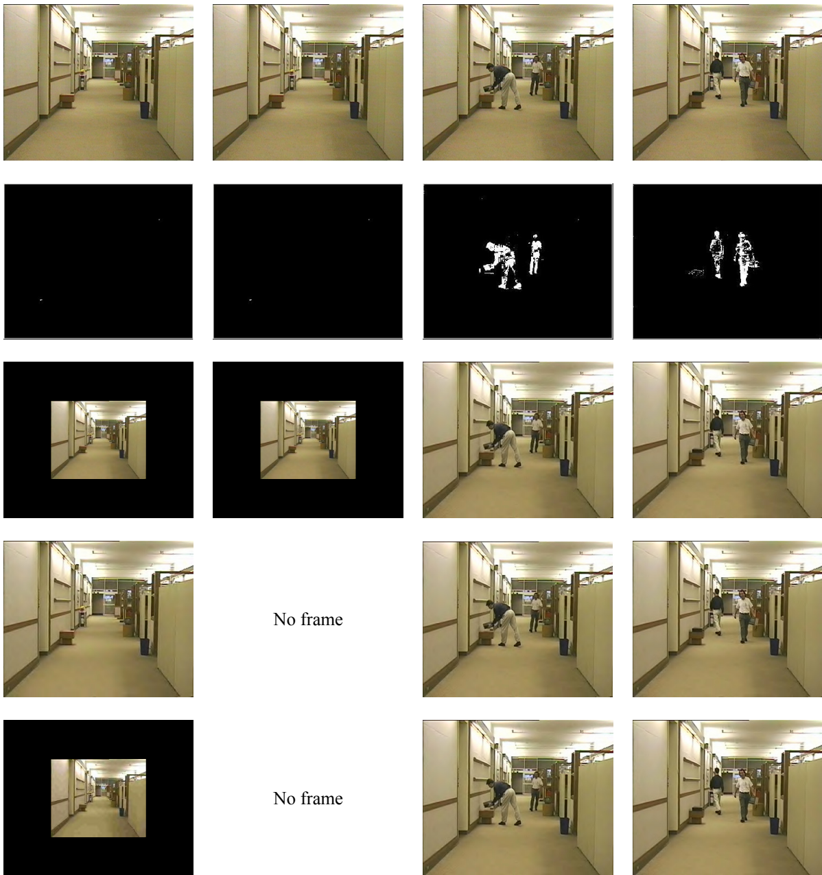
Figure 4: Frames of the reconstructed “Hall” sequence obtained. First row: the original frames. Second row: binary mask. Third row: spatial adaptation. Fourth row: temporal adaptation. Fifth row: combined adaptation.
